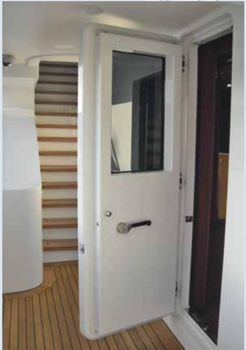
180° opening width through hidden hinges patented, made of Stainless Steel AISI 316 and polyamide with high mechanical performance, either with manual pantograph stainless steel AISI 316 arm or electric.
