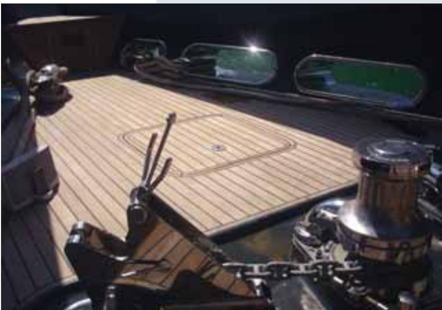
Our flushhatches which can also be prepared for the bonding of the teak, are equipped with a locking system with 4 or more polished stainless steel dogs and it can be opened from the inside through a wheel or lever and from the inside through a removable star-lock.
